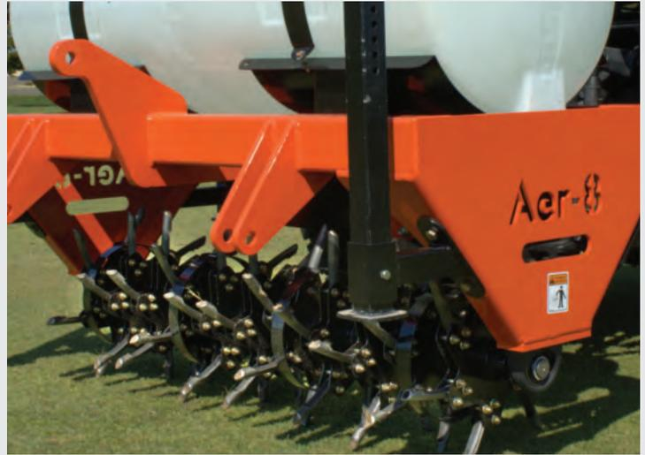
Aer-8 units are available in 60" (152 cm) and 78" (198 cm) widths, either pull-type or 3-point hitch mounted frame styles. The pull-type kit can be outfitted with hydraulic lines directly to the tow vehicle or with an electric/hydraulic power pack. The power pack includes a remote control to the driver's seat and a battery-charging cable to maintain charge in the battery through repeated use.
