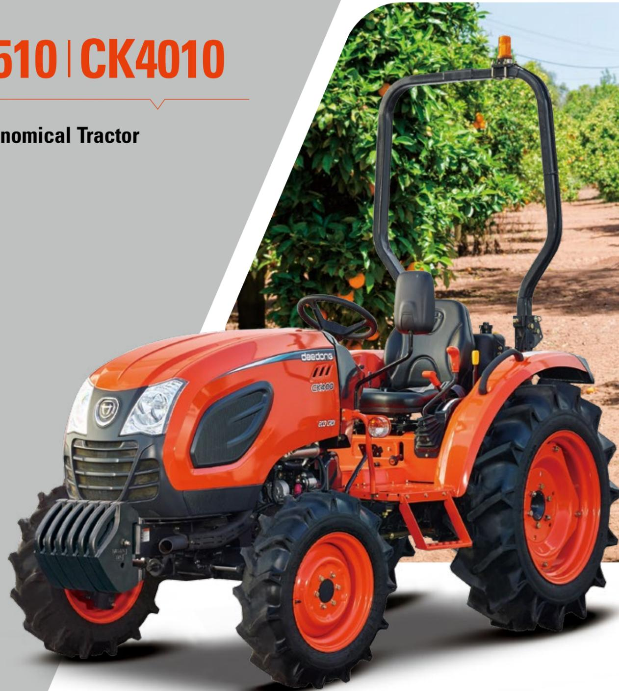
Equipped with new Stage 4/Tier 4 engines, new CK tractor provides better engine responsiveness while maintaining the best levels of fuel consumption. The extra power is thanks to the engine power management feature which automatically boosts power to increase output for a range of work taking account of PTO operation, travel speed and load.
